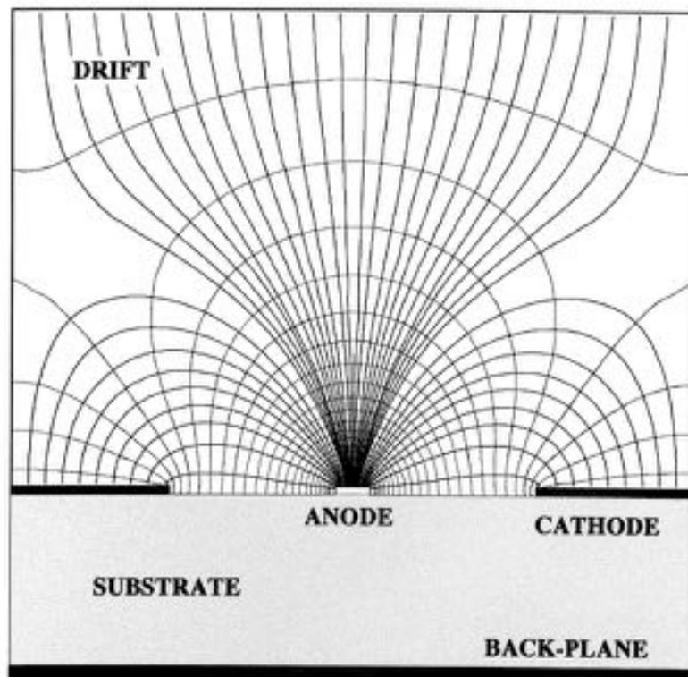
10  $\mu\text{m}$  wide anode strips, 50  $\mu\text{m}$  cathode strips at 100  $\mu\text{m}$  pitch on glass substrate:
