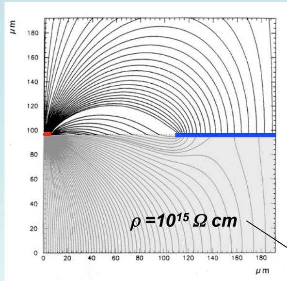
The electric field at the edge of the strips is strongly affected by the resistivity of the support:
