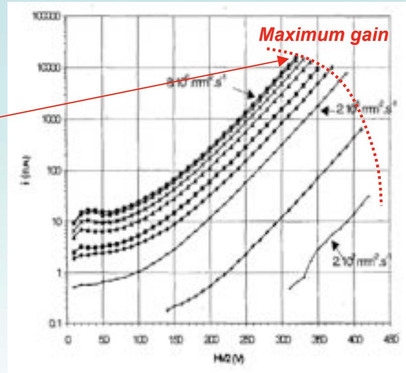
Proportionality: the current is proportional to the flux and the curves are parallel up to  $8 \cdot 10^6 \text{ mm}^{-2} \text{ s}^{-1}$ . The maximum gain depends on flux: at  $10^6 \text{ mm}^{-2} \text{ s}^{-1}$  it is about  $10^3$ .
