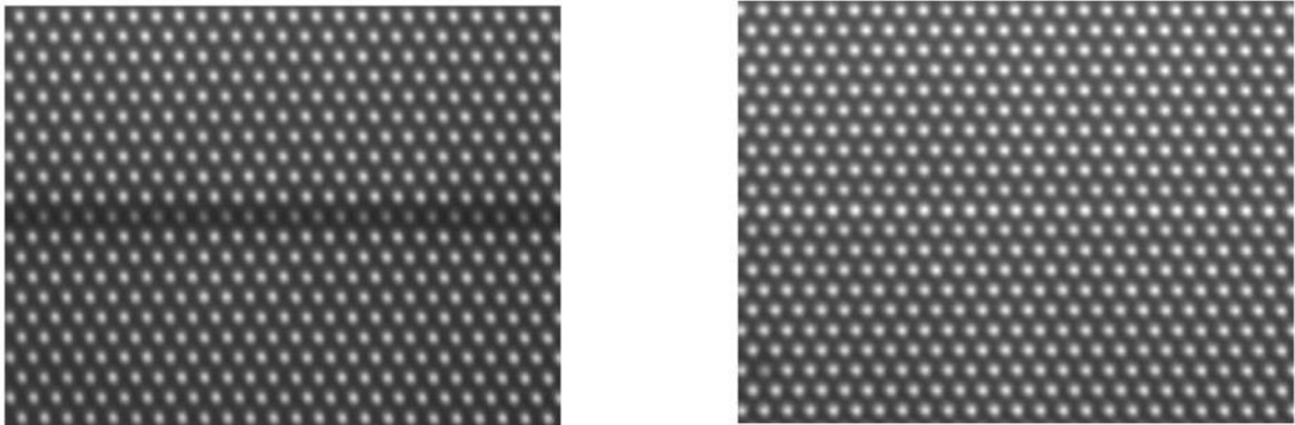
Figure 9-4: Photons emission image recorded with a GEM foil in two configurations of the sectors separation (Marques et al. , 2020).
