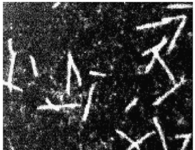
Fig. 74. Neutron conversions in ^3\text{He} recorded with a solid state camera from the photon emission in a multi-GEM amplifier.
