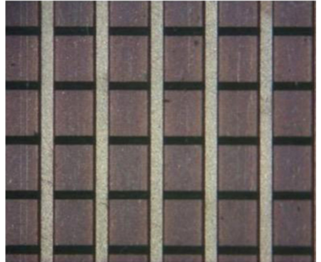
Fig. 26. Two-dimensional projective readout, with X-Y strips at 400 \mu m pitch. Top and bottom strips are 80 \mu m and 340 \mu m wide, respectively.
