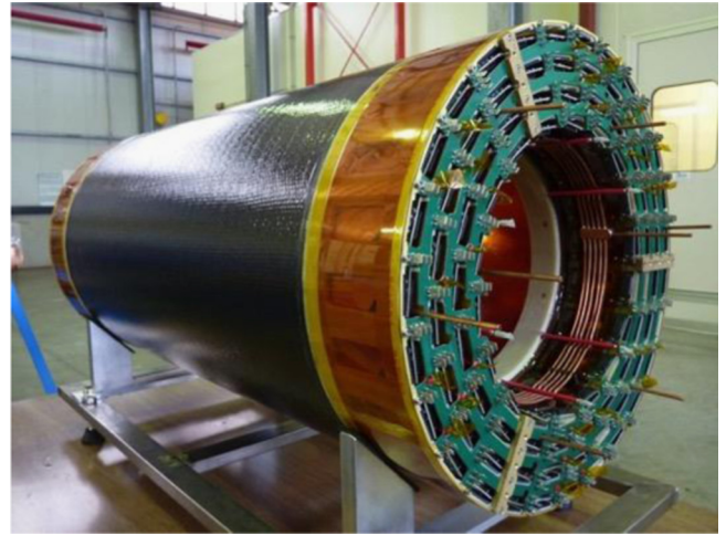
Fig. 37. The Triple-GEM tracker for the KLOE experiment, 70 cm long.
