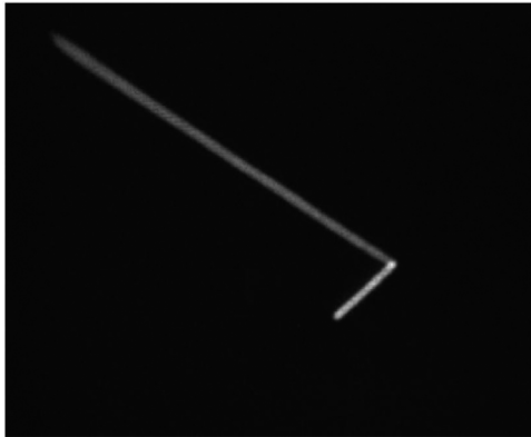
Fig. 16. A ^{220}\text{Rn} decay within the sensitive volume [34].
