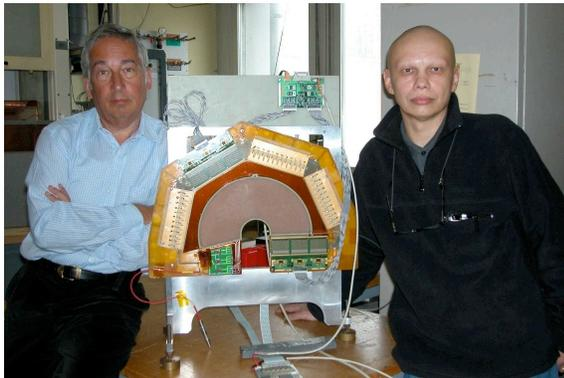
Fig. 4: Prototype of a GEM detector for TOTEM.
