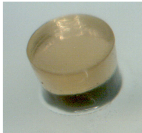
Fig. 10. Close view of an insulating pillar, 300 \mu\text{m} in diameter.
