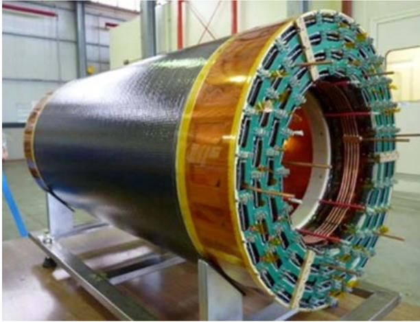
Fig. 25. Four-layer cylindrical GEM detector for the KLOE-2 inner tracker in Frascati.<sup>59</sup>
