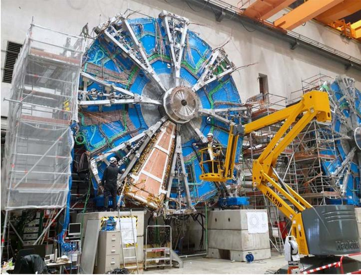
Fig. 10. Installation of a MICROME GAS-thin-gap chamber module on the NSW.
