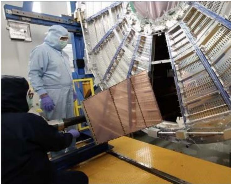
Fig. 35. A three-module GEM panel being mounted on the outer readout chamber of the ALICE TPC upgrade. *Source:* CERN, 2019.
